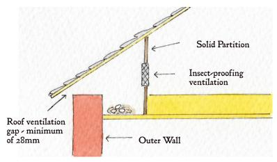
By far the easiest and most effective, this method can also be used to make a new nesting place. The swifts use the ventilation gap which is there to keep air circulating in the loft. A partition can be inserted to prevent swifts entering any further.
