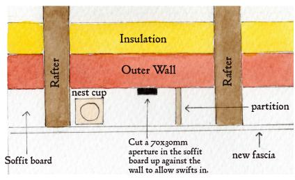
If you are having new soffits fitted, this is an ideal solution. Try to cut the entrance hole as close to the original as possible, and if you are providing more than one nest space, put partitions between them to prevent fights between birds. The nest cup helps the swifts to make a secure place for the eggs to sit.
